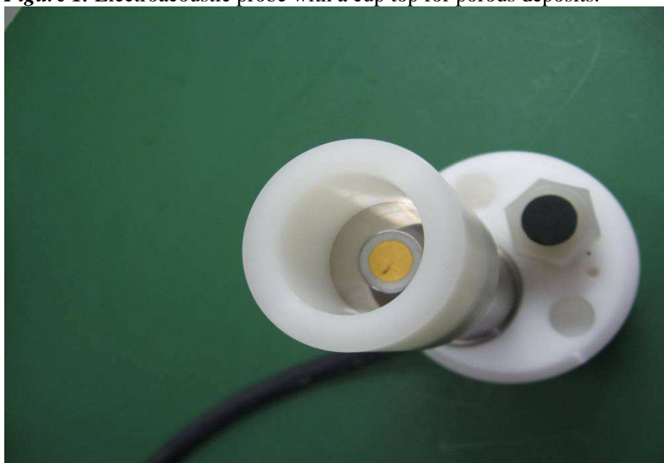
Figure 1. Electroacoustic probe with a cup top for porous deposits.
